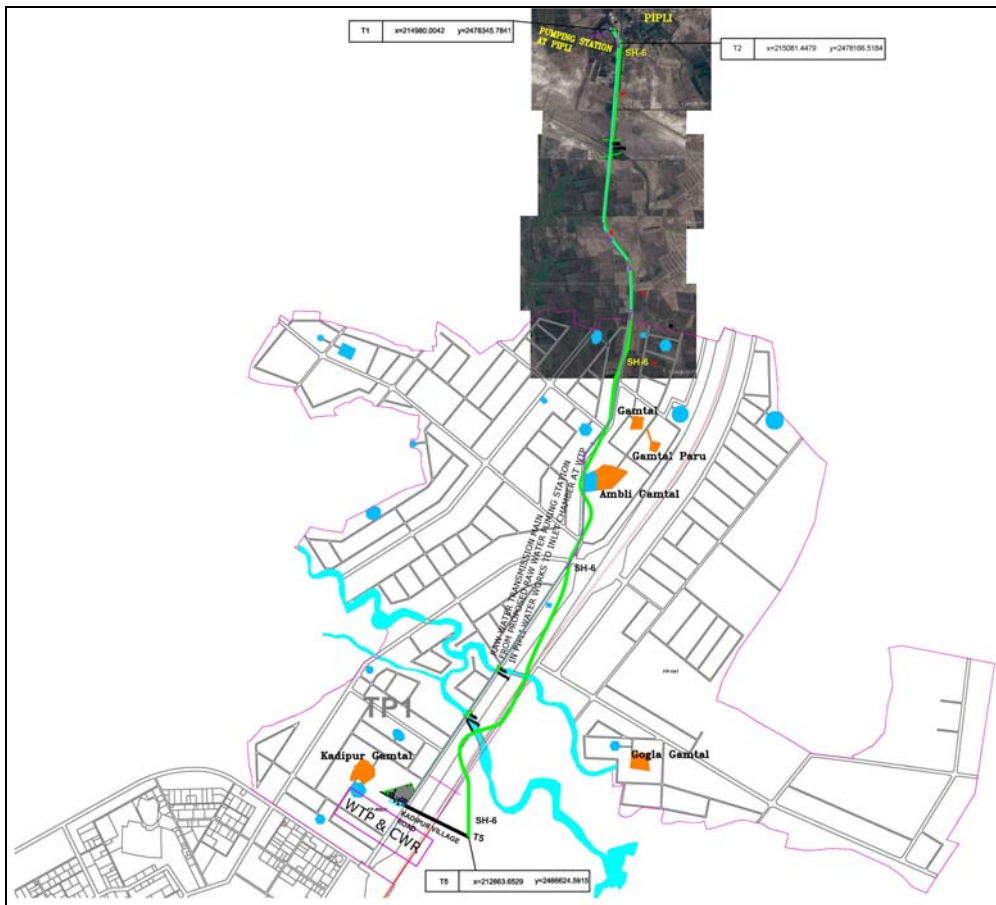
LOCATION OF RAW WATER PUMPING STATION AND ROUTE ALIGNMENT OF TRANSMISSION MAIN FROM PIPLI TO WTP
