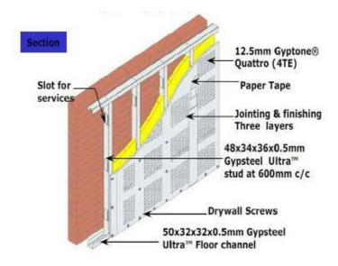
Item No: 53 - Providing and Fixing in position 50mm thick glass wool in slab form of density 24 Kg/cum of UP Twiga make or any other approved make behind wall paneling as shown in the drawings and manufacture's specification. The Installation shall be as per following steps:
